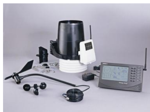
figure 9: Davis Vantage pro weather station with anemometer, tipping bucket and console displayed
