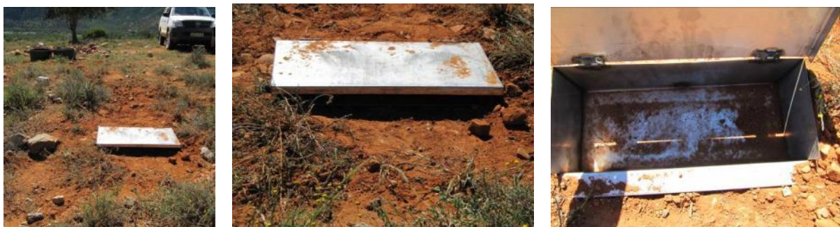
figure 10: Layout of Gerlach troughs; left: field set up, middle: close up, right: close up with Gerlach trough open, down at the bottom in the middle is a hole on which a hose is connected to one of the partly submerged steel drums under the tree visible in the left image
